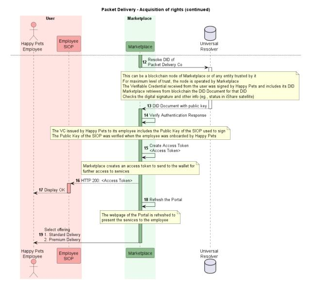
Figure 6.4.b: Sequence diagram for step "Acquisition of Rights / Activation"
