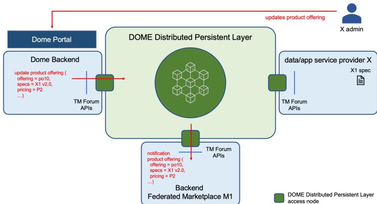
Figure 5.5 - interactions among components during reference stage
