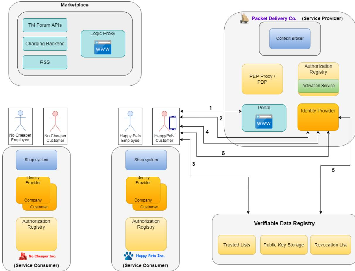
Figure 6.5.a: Architecture diagram for step "Change PTA by Happy Pets customer"
