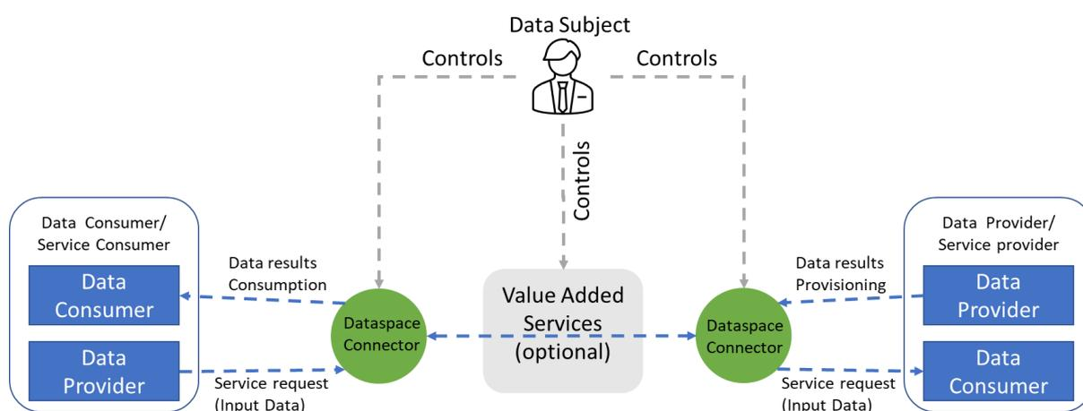
Figure 2.6 Interaction between Provider and Consumers
